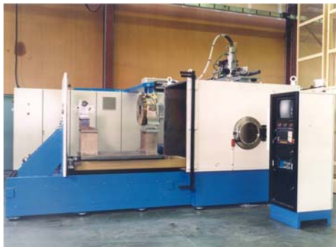
Fig. 19 :Medium size universal EBW machine
