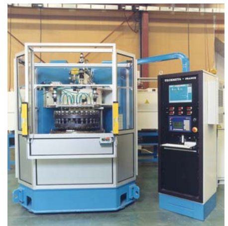
Fig. 21 :Double gun high productivity EBW machine for automotive parts
