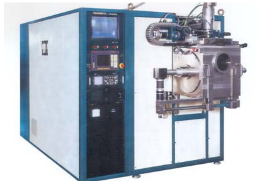
Fig. 20 :Small size universal EBW machine
